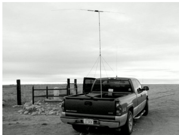
Cornhusker special with 40m and 160m resonators at WY/CO/NE
