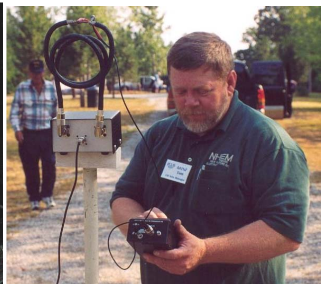
Antenna Shootout coordinator Tom Bates, AA1NZ, checks out the SWR on the receiving antenna.
