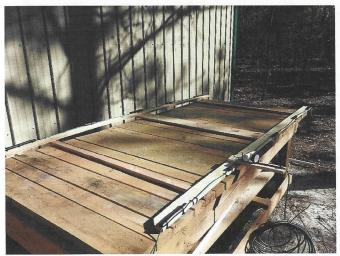
Last year I made an earlier test version of this beam with a PVC backbone. With help from Joel Hallas W1ZR (ARRL fame) I was encouraged to experiment further. Imagine a beam that's 50% reduced in length, easy to build, easily tunes 28-29 MHz and has high gain (about 7 dBi when mounted 35 ft high!). Since this would be a temporary antenna, I used whatever wood scraps I had on hand for the backbone. I used green insulated aluminum clothesline wire (9 ga.) for
