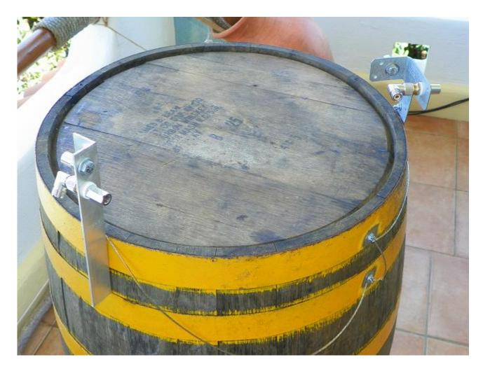
Note the old rum barrel on wheels in the photo above used as my "antenna test table" complete with antenna connectors. I bonded the first two metal rings together and to the antenna connectors to broaden the ground plane.
