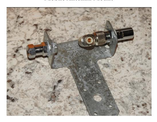
Easy to make and heavy duty. You can spend \$10-\$20 on one or make your own mobile antenna mount. A hurricane connector "Tee" (#66T) is available at your home improvement stores for about \$4.00. Bend the ends 90 degrees and drill a hole to accept the antenna connectors. Rotate for a vertical or a horizontal dipole and bolt/screw to your mast.
