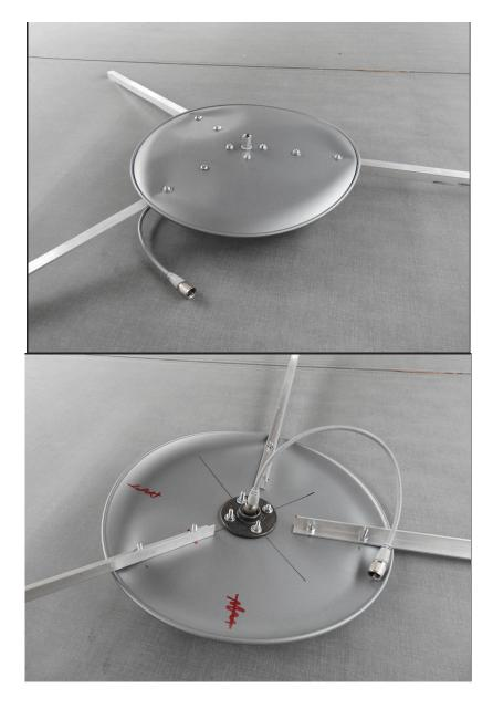
Using a pizza pie tin and 3 pieces of scrap aluminum angle (tubing works too) and a few  $\frac{1}{4}$ " bolts. Drill holes and mount a  $\frac{3}{4}$ " pipe stand fitting. Install the 3 ground radials (to broaden the ground plane), slide the coax through the pipe mast (your length using  $\frac{3}{4}$ " threaded pipe), connect the coax and screw the mast to the pipe stand fitting over the PL-259 coax connector.
