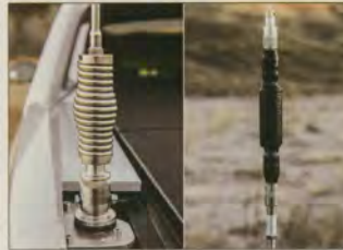
Figure 3 — Close-ups of (left) optional base spring, and (right) the completed loading coil.
