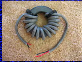
Type 31 Toroid for motor control leads
