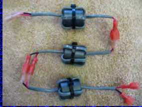
Type 31 Beads X3 with Motor Control Leads
