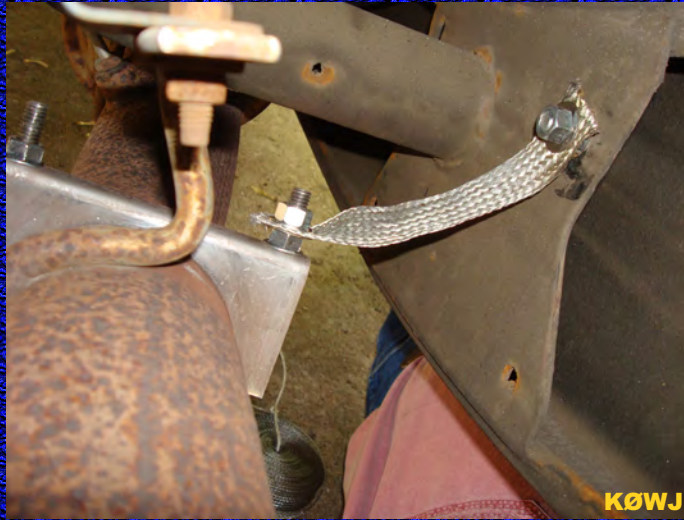
Exhaust Pipe Bonding
