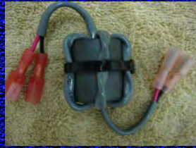
Type 31 Bead for motor control leads
