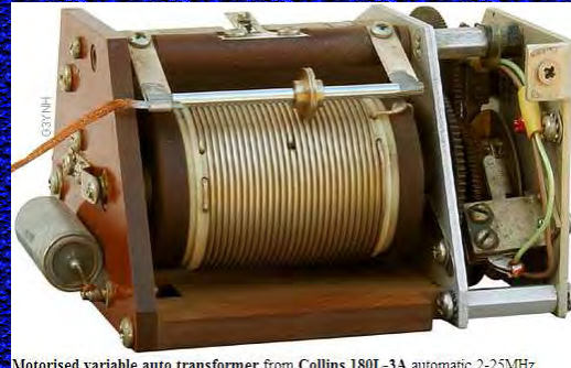
Motorised variable auto transformer from Collins 180L-3A automatic 2-25MHz
