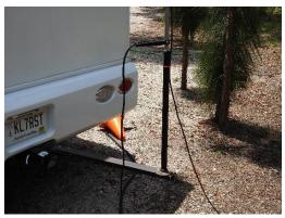
I'm testing which antenna mount works the best. Didn't have many choices, hi hi! Pictured is a 1.5 inch angle iron by 3 foot long bolted to the hitch (less ball). I also grounded the mast to the frame. With more permanent supporting this
