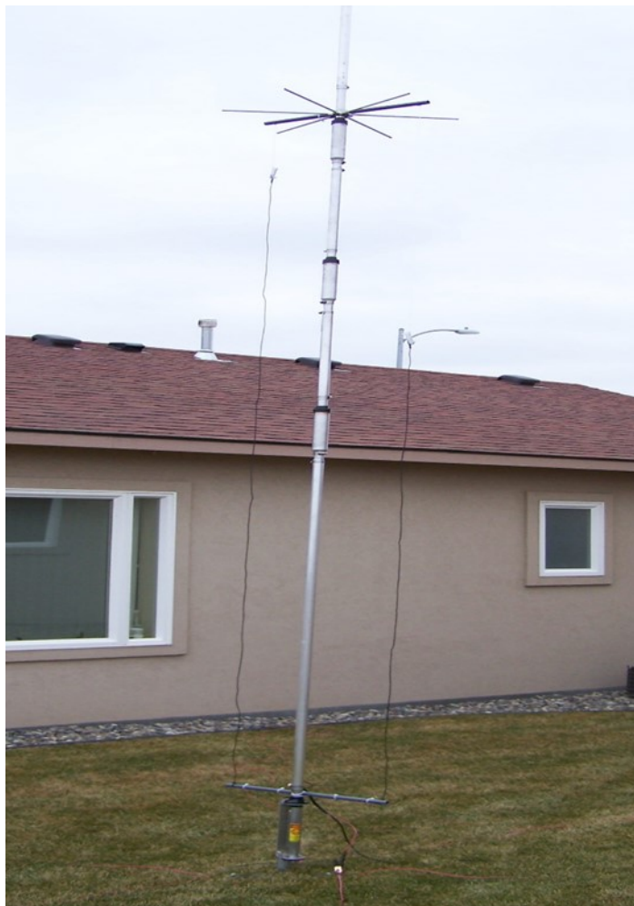
Finished "mod" showing 12 and 17 Meter add on verticals
