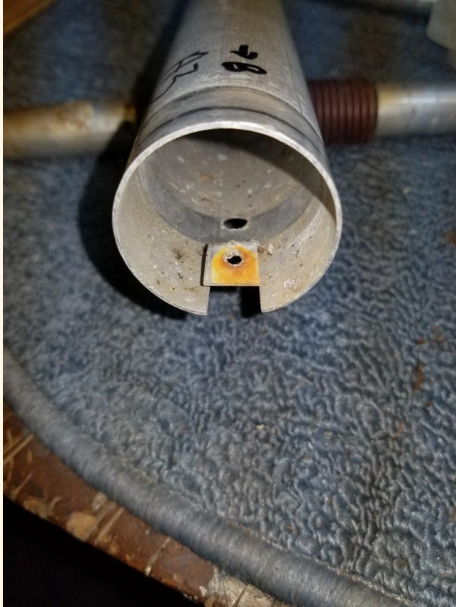
15. Close up of the tab end of the tube and you can see inside the tube where the nylon spacer was situated originally.
