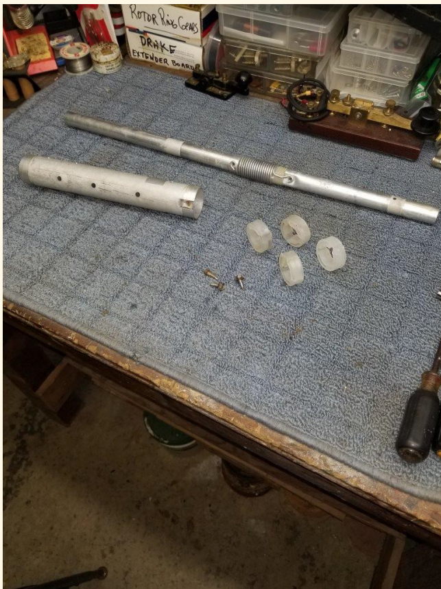
16. All the innards of the 10M trap. Especially notice the sheet metal screws. #6 and #8 with external lock washers. Every screw, washer, nut and bolt was replaced with 80-8 stainless steel. Every connection was cleaned with scotchbrite pads or brass bristle brushes and then a Penatrox A type corrosion compound (compatible with copper, aluminum, and stainless connections) was used to coat the contact areas with a thin film.
