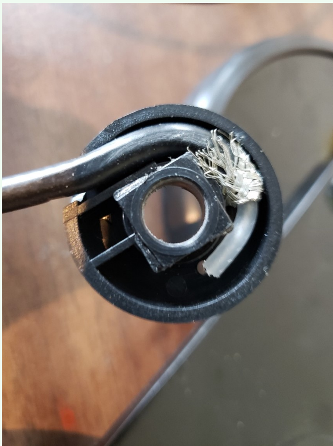
Example of antenna connection, again compression contact
