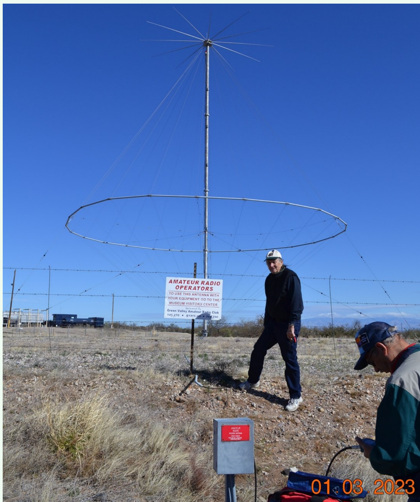
KU1V, Gray box is the antenna connection point
